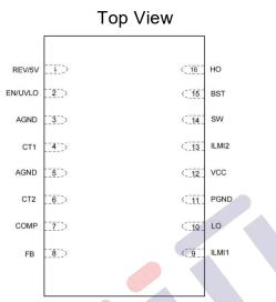
Connect Exposed Pad on bottom to AGND and PGND on the PCB
